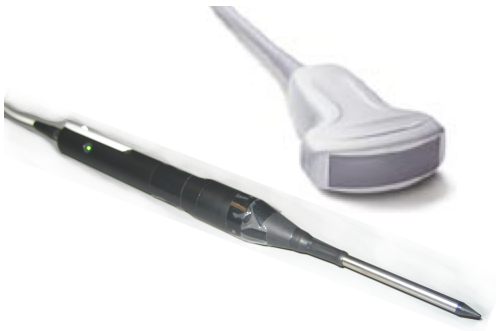
Figure: Ultrasound transducer and tracker probe
