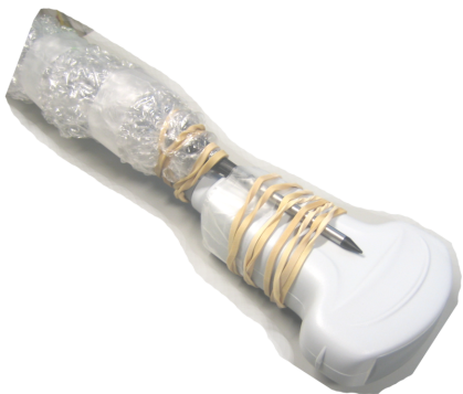
Figure: Ultrasound probe with attached tracking sensor
