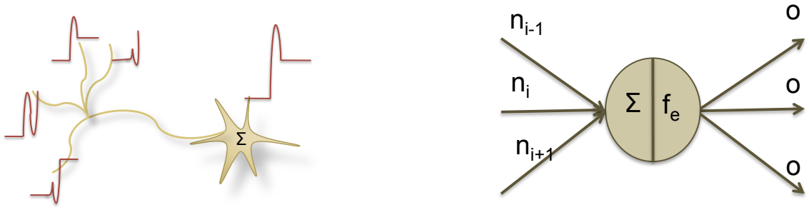
Figure 2.1: A perceptron (left), computing unit of ANN, can be analogous to a biological neuron (right). Like a biological neuron exchange its signal in the form of potential, a perceptron does with numerical values.
