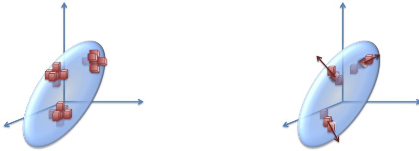
Figure 3.3: A neighborhood system comparison between a traditional (left) and an adapted (right) system: A traditional neighboring system considers 8 directions regardless of structures position while the adapted system here considers only two along the gradient descents direction of structure priors.
